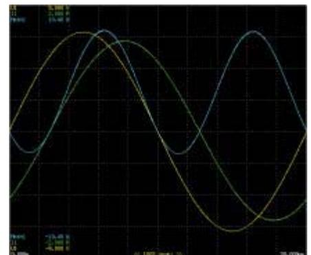
Figure 2: Power signal (blue) calculated from  $u(t)$  (yellow) and  $i(t)$  (green)
