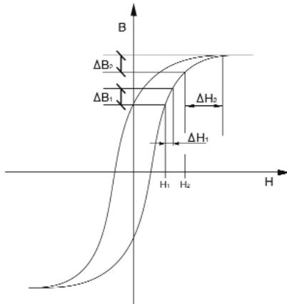
Figure 10: Hysteresis cycles of the magnetic cores
