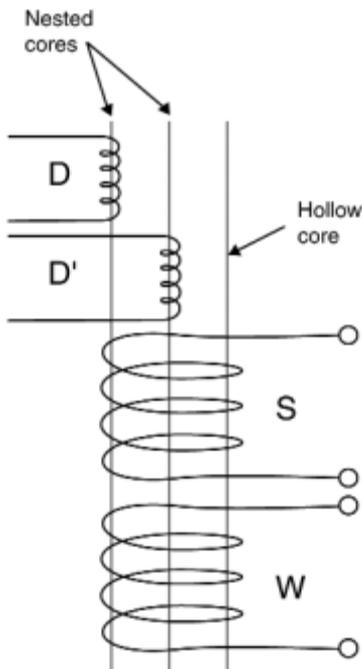
Figure 14: The various windings used and their arrangements
