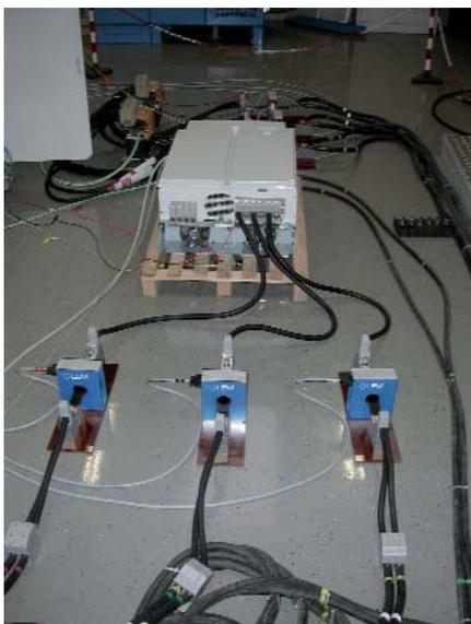
Figure 1: Six channel power measurement at KEB inverter
