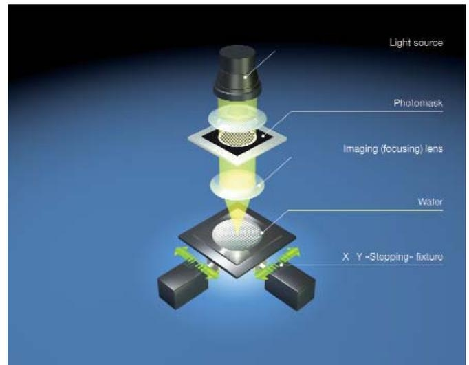
Figure 7: The basic principle of photolithography
