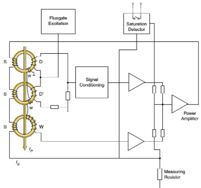
Figure 16: ITxx operation principle: simplified overall diagram
