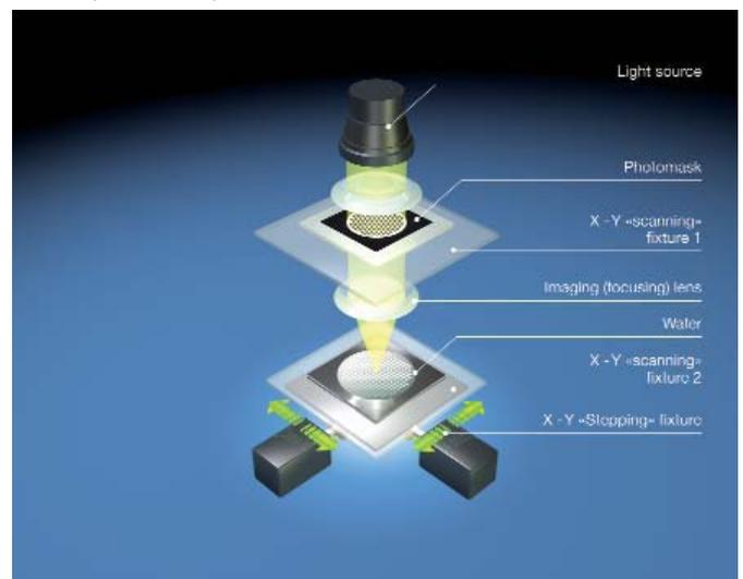
Figure 8: The photolithographic scanning stepper
