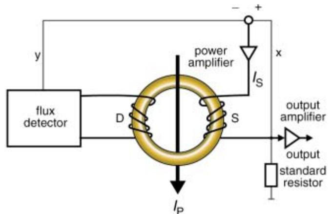
Figure 12: Simplified base circuit for DC current compensation
