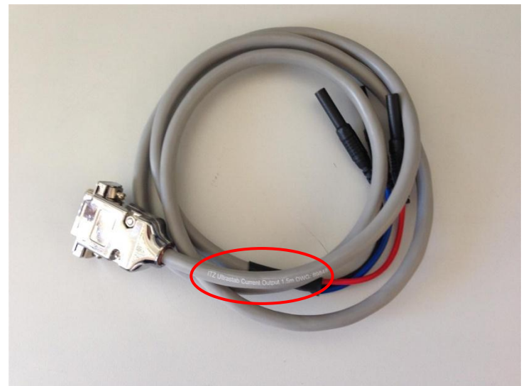
D-SUB-cable „ITZ ULTRASTAB CURRENT OUTPUT“ for current output
