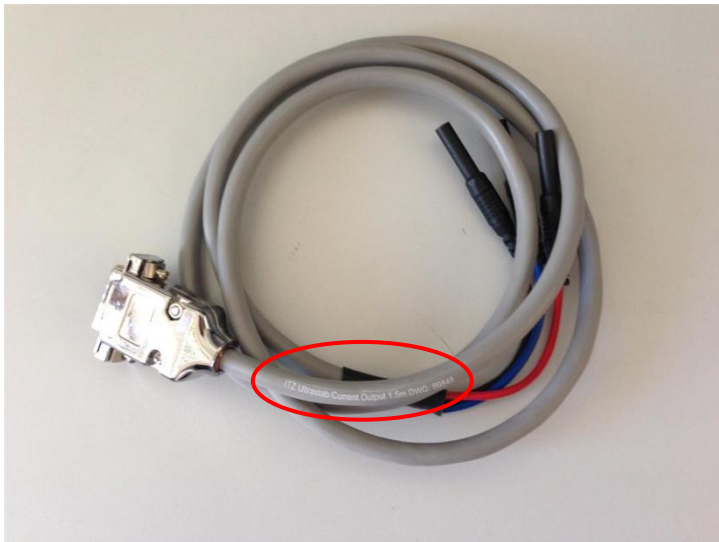
D-SUB-cable „ITZ ULTRASTAB CURRENT OUTPUT“ for output current
